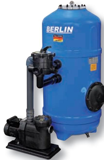
with 4-way nozzles, a drain cock including a hose connection, pressure gauge and manual air bleeder. The customized equipment is compatible, e.g. manual or automatic 6-way backwash valves and rod valves. An ozone-resistant finish, nozzle base, sight glass and a manhole with an acrylic glass cover can be realized depending on the customer's requirements
